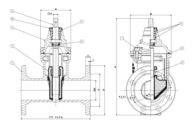
Figure 1: Gate valve cross-sectional drawing
